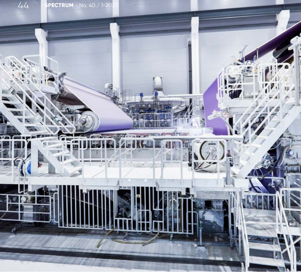
The forming section is equipped with a hybrid former.
